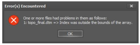
This error message is caused by trying to import a Surpac DTM in binary format
